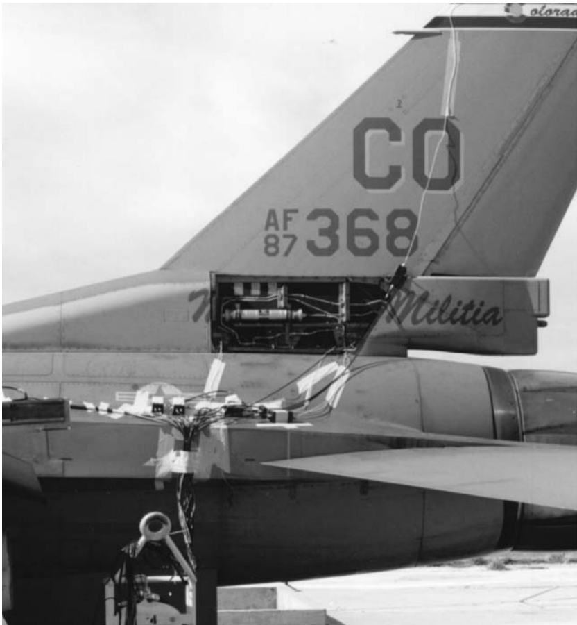
FIGURE 6.36 Instrumented F-16 for engine noise tests.
