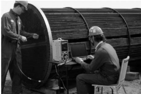
FIGURE 5.51 Demonstration of RFT on a tube bundle extracted from a heat exchanger. The technician on the left is pulling the RFT probe, while the technician on the right operates the instrument, storing examination data by tube name. Only the tubes on the outside of the bundle can be examined visually; hence the need for RFT. The thick circular plate where the ends of the tubes are visible is called the tubesheet. The thinner plates further to the right are the tube support plates. (Courtesy Russell NDE Systems.)
