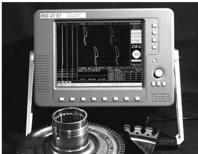
FIGURE 5.55 Eddy current inspection of a turbine disk. Note this particular system displays the response of a specialized probe with four eddy current sensors. (Courtesy Zetec, Inc.)
