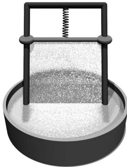
FIGURE 2.2 Classic experiment to demonstrate the details of surface tension of a fluid.
