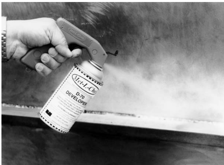
FIGURE 2.15 Picture of developer being sprayed onto specimen. (Courtesy Met-L-Chek.)
