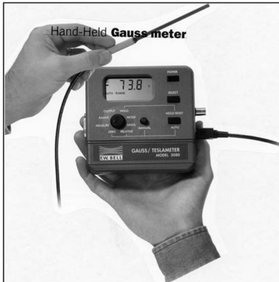
FIGURE 4.36 Gauss meter used to measure the strength of the magnetic field.
