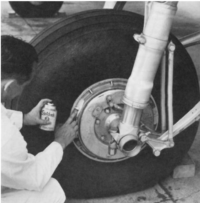
FIGURE 1.3 Penetrant testing applied to a safety critical part on an aircraft—the landing gear. (Courtesy Magnaflux.)
