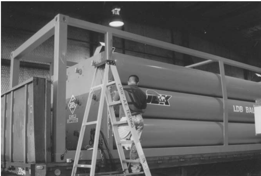
FIGURE 6.23 A tube trailer being instrumented for an acoustic emission requallification test. (Courtesy of City Machine and Welding, Inc., Amarillo, TX).
