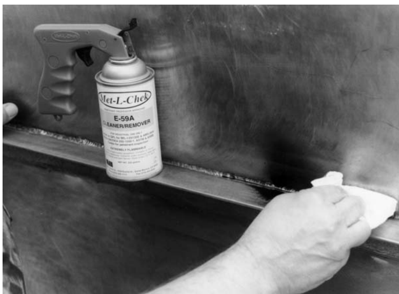
FIGURE 2.14 Picture of cleaning excess penetrant from specimen surface. (Courtesy Met-L-Chek.)
