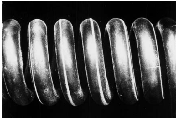
FIGURE 4.42 Deep seams in coil spring.
