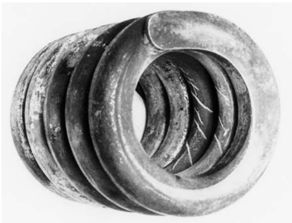
FIGURE 4.43 Fatigue cracks in coil spring (45° from long axis).
