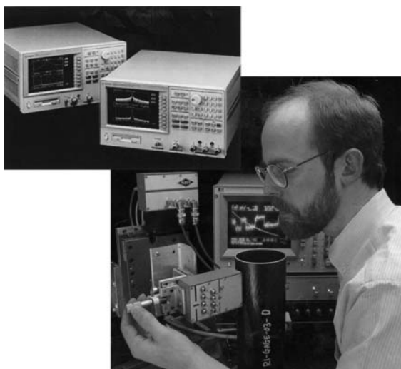
FIGURE 5.36 Eddy current measurements on graphite-epoxy tubing using a network/impedance analyzer. (Courtesy Hewlett-Packard.)
