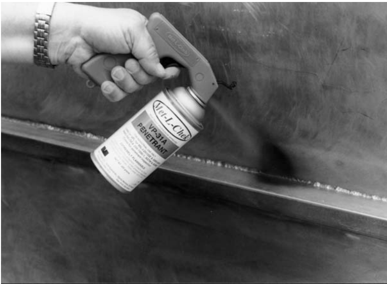
FIGURE 2.11 Picture of visible penetrant being applied. (Courtesy Met-L-Chek.)
