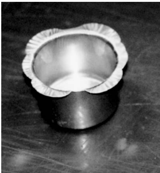
FIGURE 1.1 Earing caused by improper texture in rolled aluminum sheet during a deep draw process for can manufacturing. In this process the NDE inspection data is used as feedback data to adjust the processing of the sheet aluminum.
