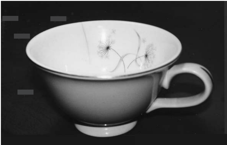
FIGURE 2.1 Crack in a coffee cup made visible by the coffee penetrating into the crack. The high contrast between the penetrant (the coffee) and the white cup makes the fine crack clearly visible.
