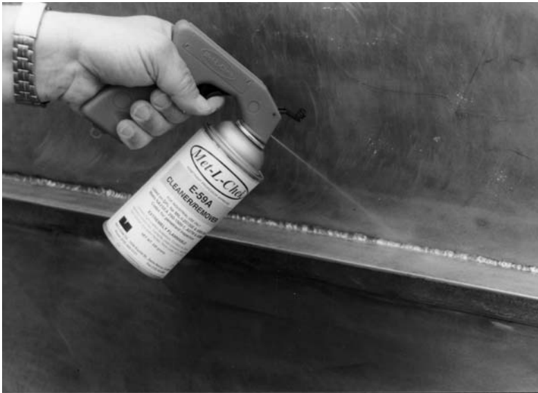
FIGURE 2.10 Picture of precleaning a specimen. (Courtesy Met-L-Chek.)
