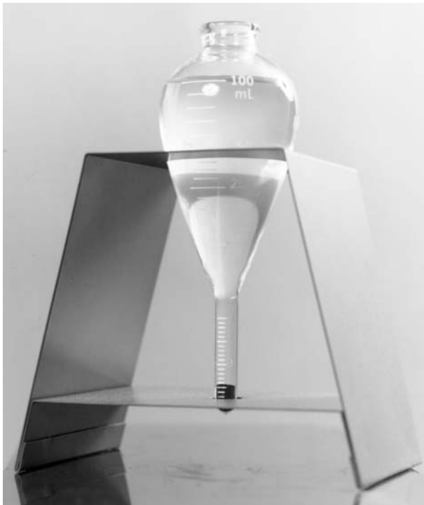
FIGURE 4.34 Centrifuge tube used to test particle concentration.
