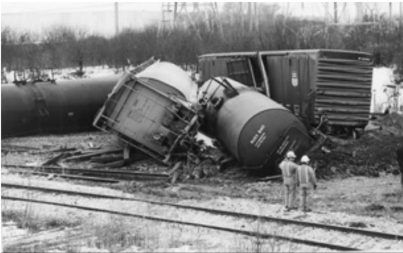
FIGURE 3.60 Possible result of a failed railroad wheel.
