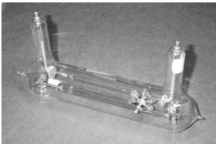
FIGURE 7.5 Cathode ray tube. (Courtesy of Oak Ridge Associated Universities.)
