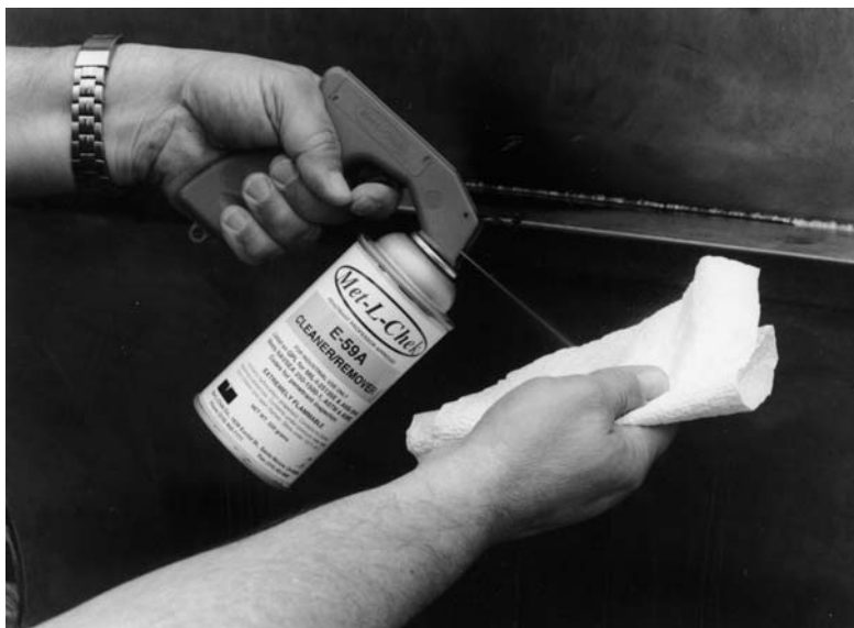
FIGURE 2.13 Picture of putting cleaner/penetrant remover on clean toweling. (Courtesy Met-L-Chek.)
