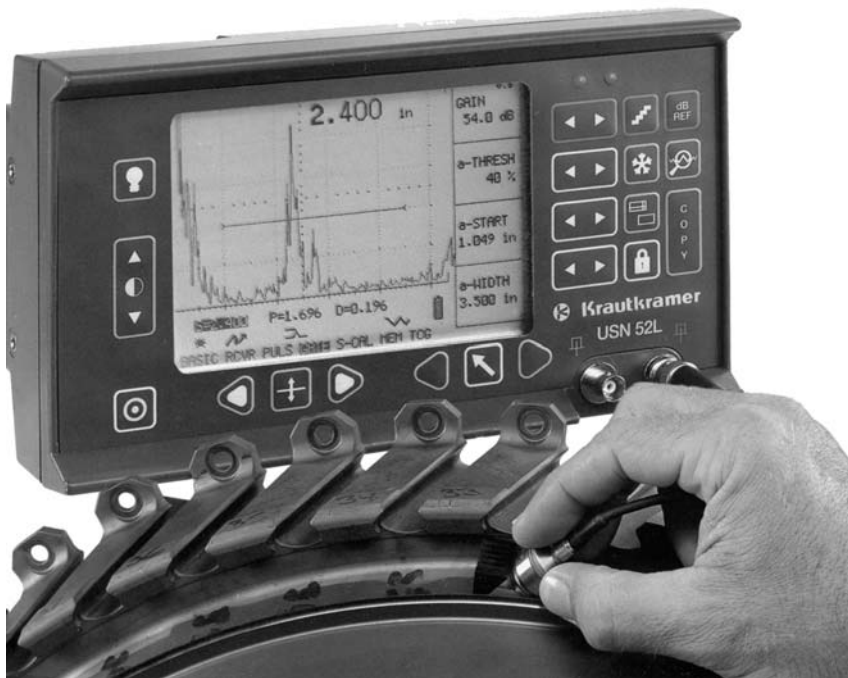
FIGURE 3.58 Typically oscilloscope display on an ultrasonic pulser-receiver system configured in pulse–echo mode. Notice the main bang. (Courtesy Krautkramer Branson.)
