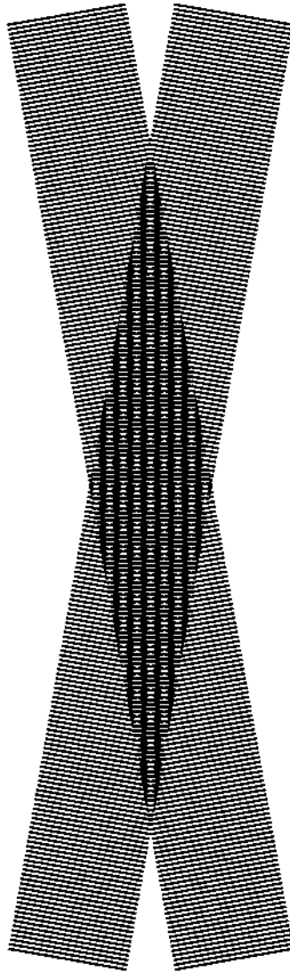
FIGURE 10.43 Moiré produced from crossed Ronchi gratings.
