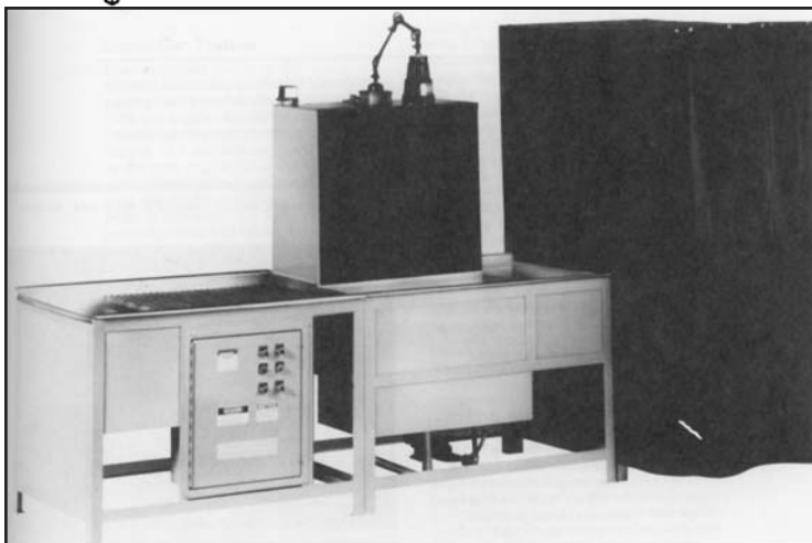
FIGURE 2.8 Schematic and photograph of a commercial liquid penetrant testing system. (Copyright 1999 © The American Society for Nondestructive Testing, Inc. Reprinted with permission from The Nondestructive Testing Handbook, 2nd ed. Principles of Liquid Penetrant Testing.)
