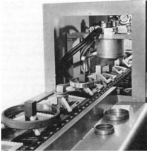
FIGURE 4.27 MPI assembly line inspection using magnetic induction method.
