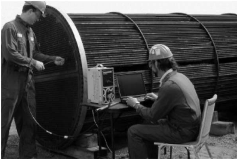
FIGURE 1.4 Partial inspection of a heat exchanger tube bundle. (Courtesy Russell NDE Systems.)
