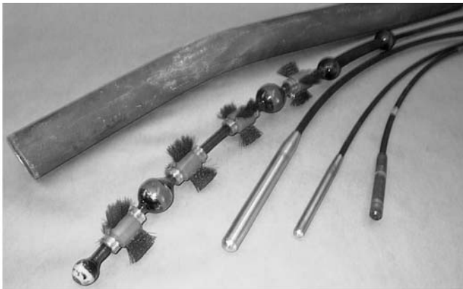
FIGURE 5.52 Typical RFT probes. The flexible probe (with centering brushes, left) is suitable for examining boiler tubes with bends, such as the sample tube in the figure. The two wear-resistant rigid probes with stainless steel casing (center) could be used to examine heat exchanger tubes. The probe without a casing (right) reveals the coil layout. (Courtesy Russell NDE Systems.)
