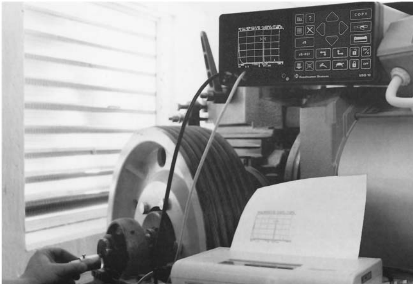
FIGURE 3.66 Photograph of UT inspection of drive shaft. (Courtesy Krautkramer Branson.)
