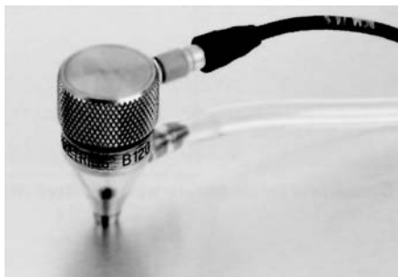
FIGURE 3.37 Bubblers use a column of continuously flowing water to couple the ultrasound between the sample and the transducer. (Courtesy Panametrics.)
